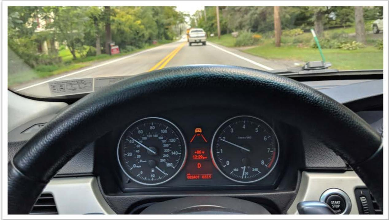
This is a very rare option from the factory as it was an over \$2,000 standalone option. The hardest part of this entire job was finding all of the parts. You will need a six-cylinder powered E9X with cruise control + brake function. This was done on a 2006 BMW 330i with an LDM module. The LDM came with option \$544 on pre-2007, six-cylinder cars.
