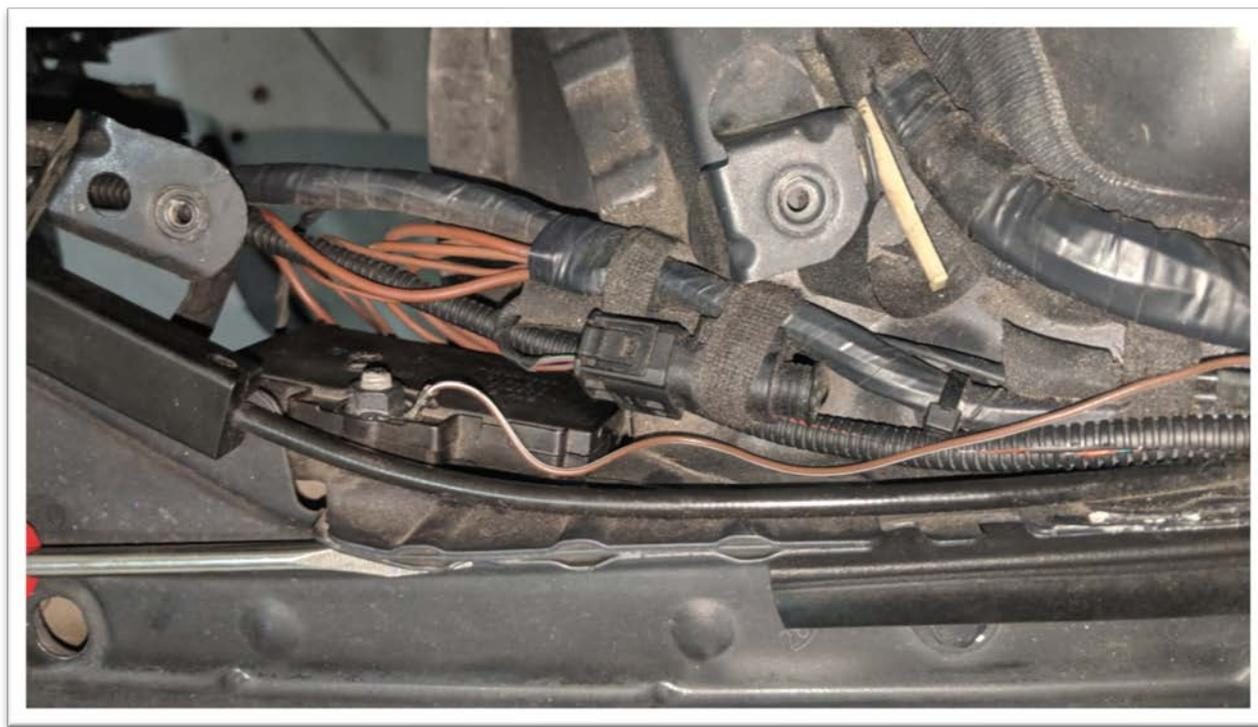
Run the harness all the way to the rubber gromet behind the DSC module. I poked a small hole through the rubber and ran the wires through. You will need to remove the driver's side under panel. I ran power from my deleted cigarette outlet but you could also run power from the fuse box. It needs to be from a 10-amp fused power source with 18-gauge wire. Pin in the signal wire to the CAS and tap the P Can lines from the LTM. I used heat shrunk butt connectors to tap the P can lines.
