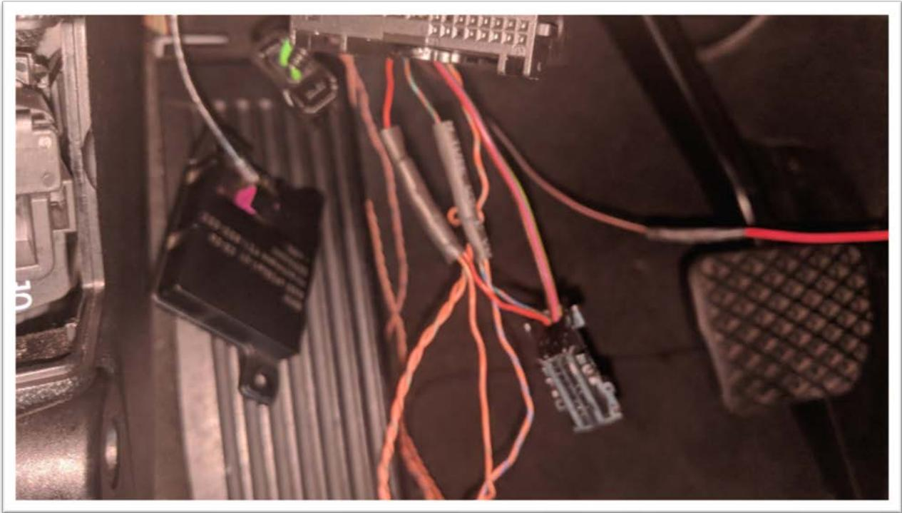
Neatly route the wires and reinstall the under panel. I zip tied the wires to the main wiring harness.
