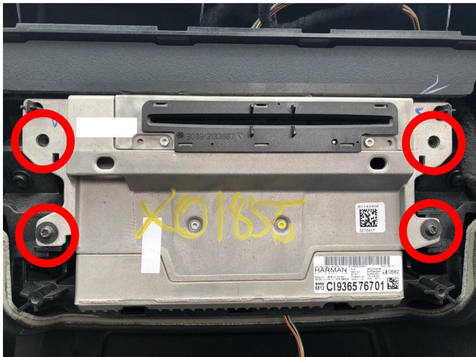
12. Remove head unit partially from the dash so that you can access the cables on the back of the head unit.
