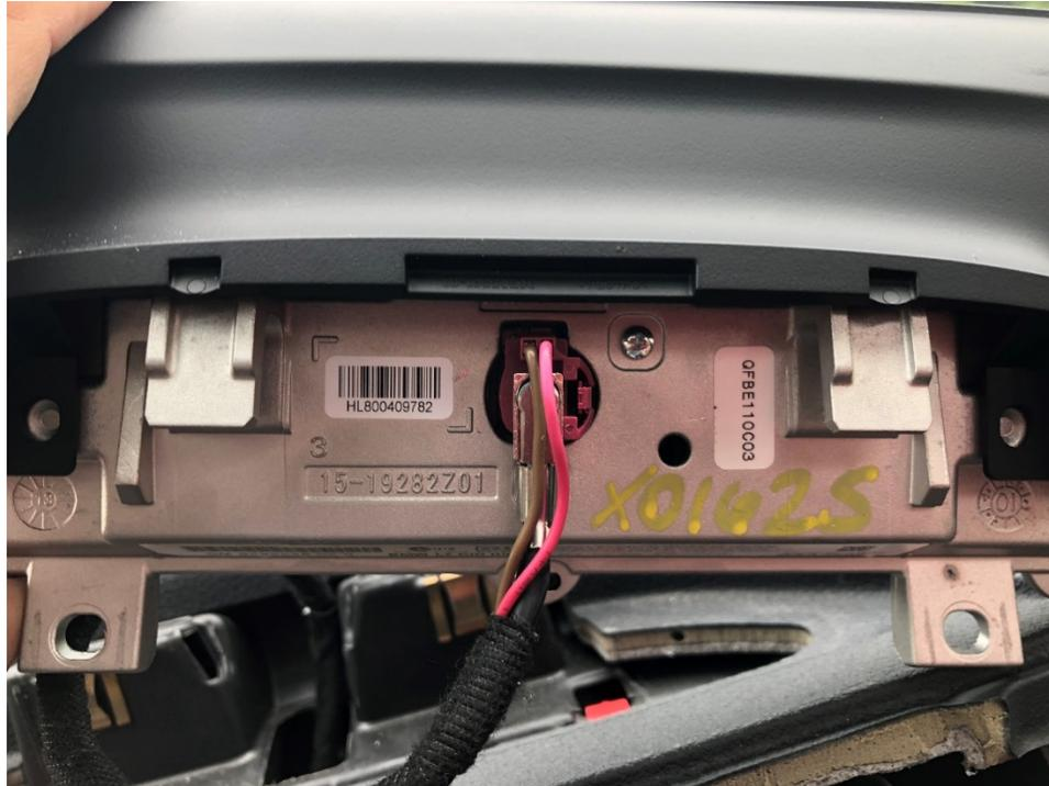
11. Remove the 4 screws holding the headunit in the dash.
