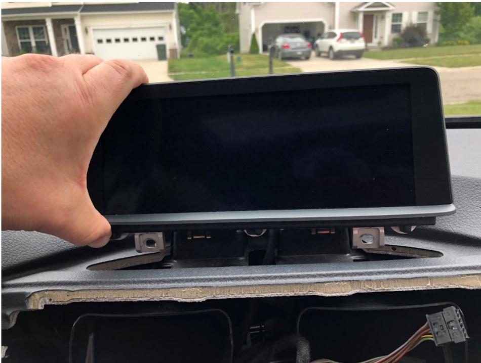
10. Disconnect the video cable on the back of the screen
