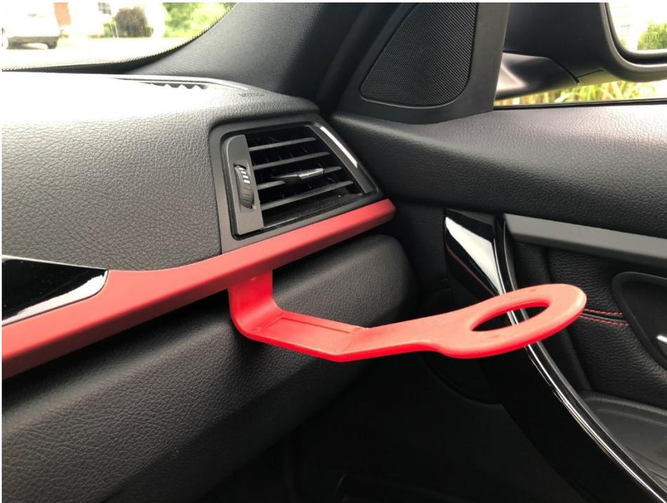
3. Pull the trim free from the dash to access the connectors behind the trim, between the vents.
